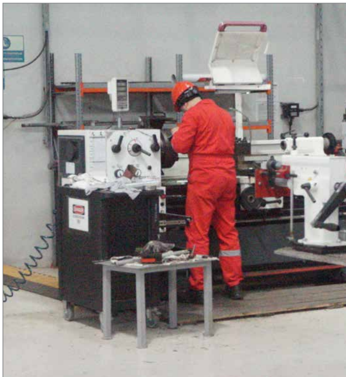
A turner preparing a special tool in the turning machine for installation of a bearing during overhaul of the C-2801 dry screw compressor
