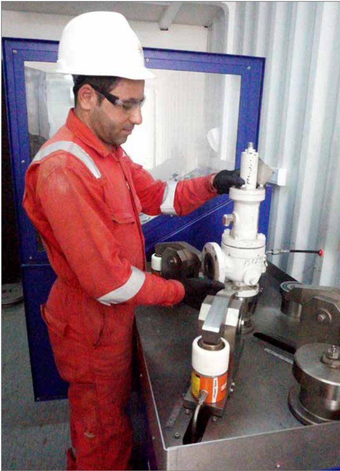
Recalibration of pressure safety valves (PSVs)
