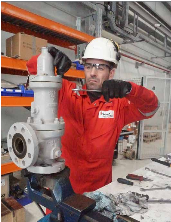
Pressure Safety Valves repaired in the workshop
