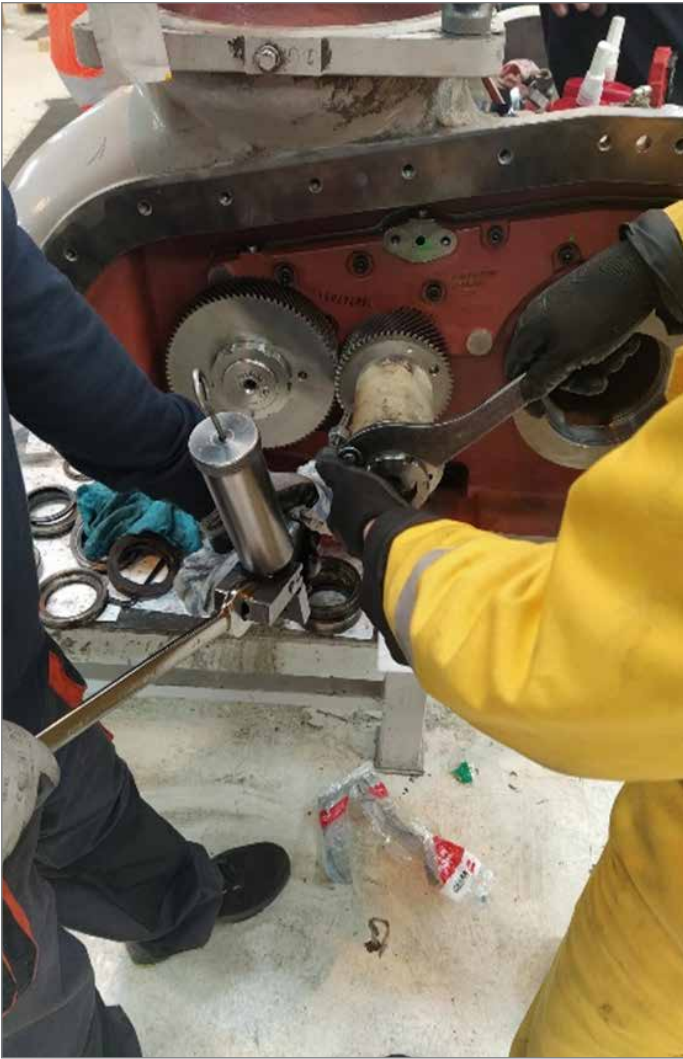
The C-2801 dry crew compressor was overhauled for preventative maintenance. The vendor (Aerzen company, Turkey) disassembled the compressor, inspected it, replaced the recommended part, and boxed the compressor up
