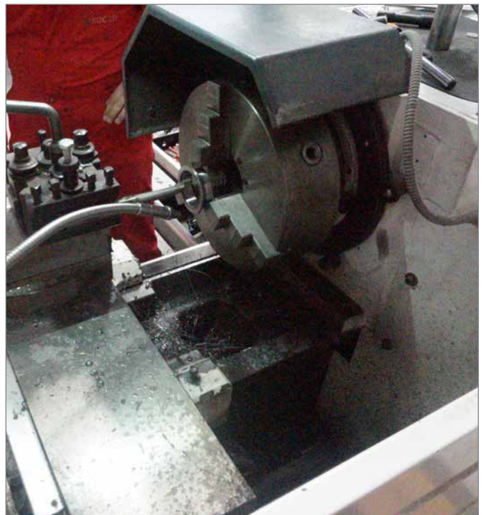
A turner preparing a special tool in the turning machine for installation of a bearing during overhaul of the C-2801 dry screw compressor
