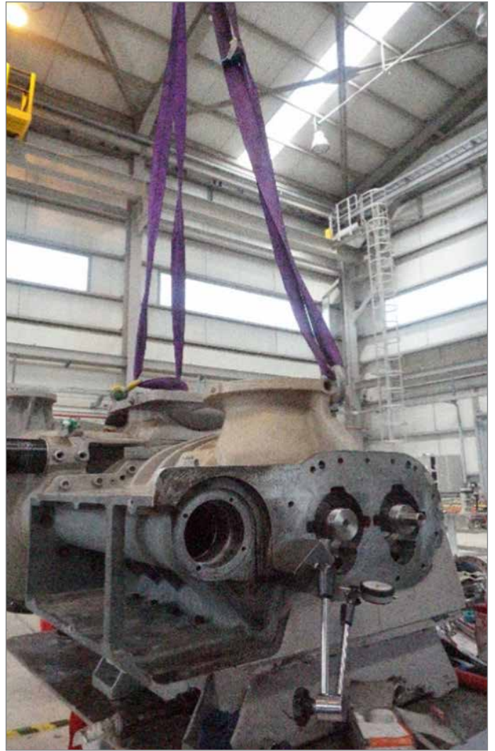
The C-2801 dry crew compressor was overhauled for preventative maintenance. The vendor (Aerzen company, Turkey) disassembled the compressor, inspected it, replaced the recommended part, and boxed the compressor up
